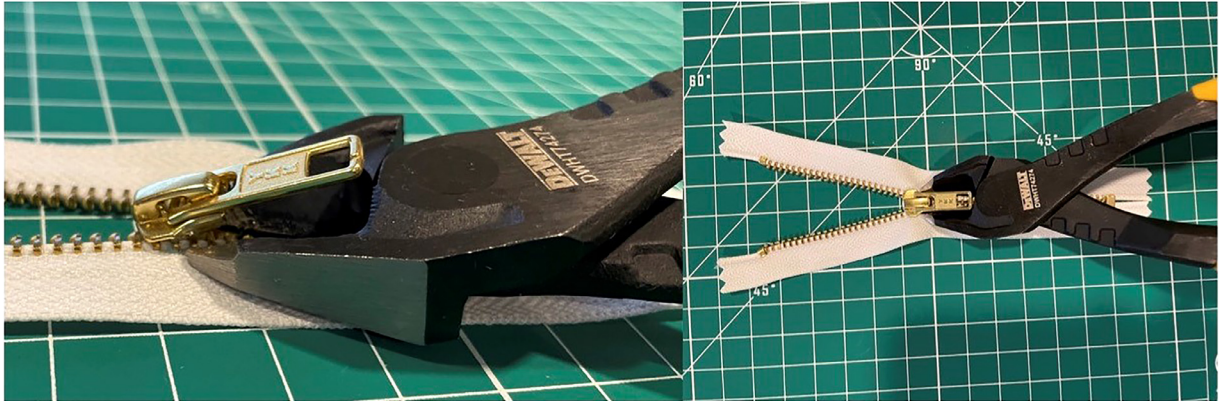
Figure 2. The wire cutters are directed towards the inferior aspect of the zipper pull and target the space between the top and bottom plates of the zipper.
