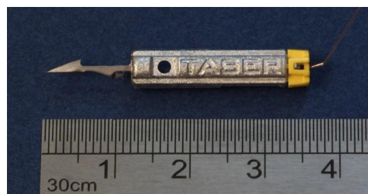
Figure 1 TASER X2 probe: a one-piece projectile.
